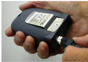
Attach the lamp cord by pushing the connector into the socket
