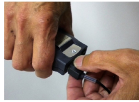
Push the connector's latch to the bottom when detaching the cord
